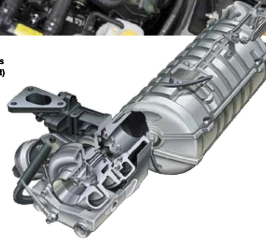
The second-generation boxer diesel boasts several new features including a new DPF system (right)
