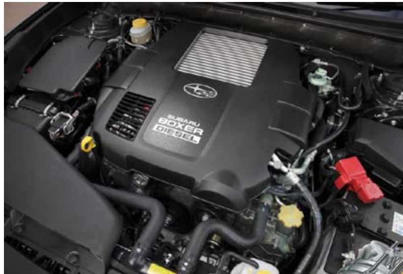
The second-generation boxer diesel boasts several new features including a new DPF system (right)
